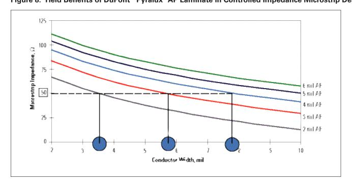
Figure 8 illustrates the fabrication benefits of thick DuPont™ Pyralux® AP flexible circuit materials core (vs. standard 2 mil) in a nominal 50 y impedance microstrip circuit. Copper traces with 2x greater line/space resolution can be used to achieve identical electrical performance while greatly reducing fabrication yield loss from fine line imaging.
